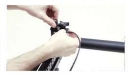
Loosen the belt clamp and insert the belt with the teeth facing down. Tighten knob to secure.
