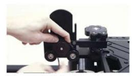
Weave the belt through the motor mount pulleys as shown.
