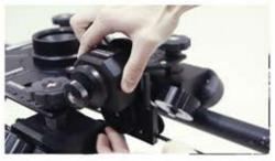
Drag module can be mounted by wrapping belt around pulley as shown and tightening knobs in back to secure.
