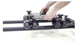
Set the assembled cart onto the rails with the truck wheels all parallel to the rails.
