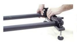
Insert the rails into the end clamp openings.
