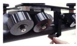
...until the bottom roller wheels barely touch the bottom of the rail. Tighten the knob. Adjust roller wheels horizontally to fit the rails. Tighten the bolts to secure.
