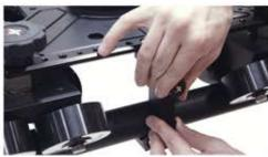
Line up the groove on the keeper arm without break with the grove on teh t-bracket and slide up...
