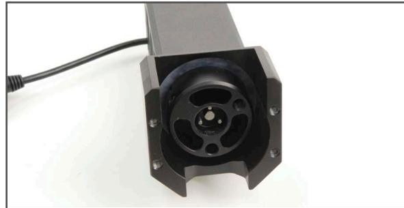
3. To install the pulley, simply push the pulley onto the motor shaft while aligning the holes. Be sure to hold the belt in place while installing.
