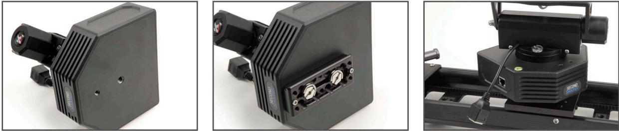
2. Connect CAT5 cable from the side of the Pan base to the PAN port on the controller.
