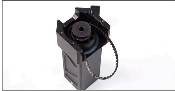
6. Mount the Slider Motor onto the Motor Mount utilizing the threaded holes nearest to the pulley on the back side of the motor.
