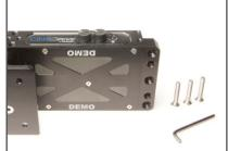
**Step 2**Remove the four Turntable Plate Mounting Screws holding the pan brick mounting plate to the pan hub. Retain screws and mounting plate for possible future use.
