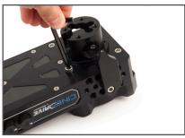
**Step 3**Re-install the top Degree Wheel.
