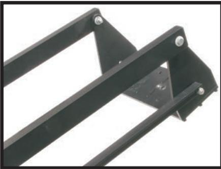
Then, flip the camera basket over and reinsert the bolts. Be sure to replace each nylon washers to their proper locations. At no time should metal ever touch metal. Proper placement of these washers will ensure smooth operation. When tightening bolts at pivot points be sure to tighten until snug then back off until pivot point moves smoothly with slight resistance. There should be no slop.
