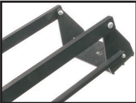
Then, flip the camera basket over and reinsert the bolts. Be sure to replace each nylon washers to their proper locations. At no time should metal ever touch metal. Proper placement of these washers will ensure smooth operation. When tightening bolts at pivot points be sure to tighten until snug then back off until pivot point moves smoothly with slight resistance. There should be no slop.
