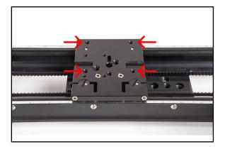
4. Use the included (4) 1/4"-20 countersunk screws and 5/32" allen wrench to mount the HD Angle Plate to the slider cart.
