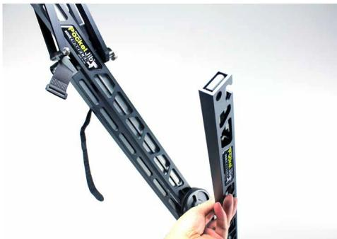
**2.** Unfold the rear arm and swing it back to align with the front arm.
