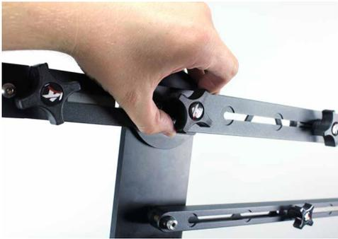
**1.** To adjust the drag on up and down movements, adjust the tension on the top knob of the jib's fulcrum point. Use this **ONLY** for drag control. It is not designed to act as a brake for an un-balanced jib.
