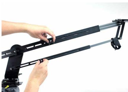
**2.** Extending the jib to desired height and tighten the knobs making sure they are seated in one of the six locking recesses.
