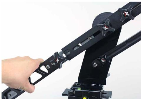
**4.** Tighten the locking knob to secure the front and rear arms together.
